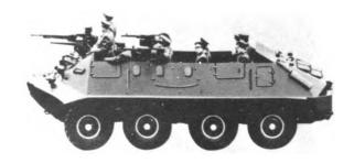
Figure 6-3. BTR-60 series eight wheeled APCs. The open-topped BTR-60P (above) is being replaced by the armor covered BTR-60PA. A newer model, the BTR-60PB (below) has a small conical turret with 14.5-mm and 7.62-mm machinegun.
